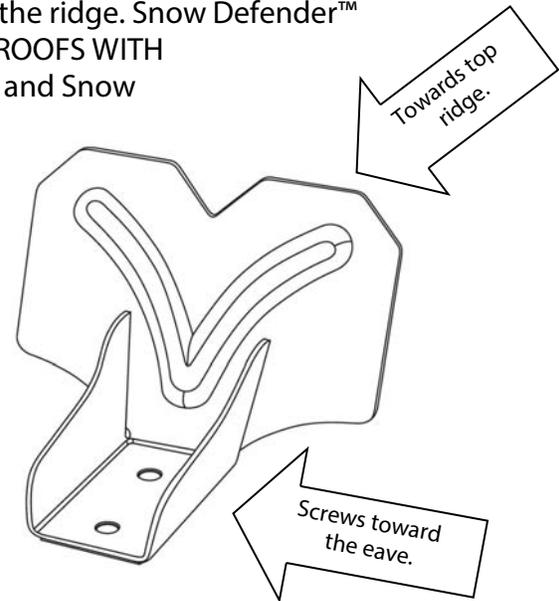
Failure to install an adequate amount of snow guards and in the proper pattern will void the warranty. Visit [www.snowdefendercalculator.com](http://www.snowdefendercalculator.com) to use our snow guard calculator to determine the amount needed.
